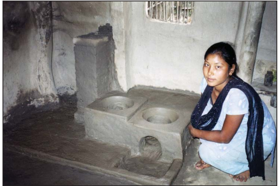
This woman is showing her newly completed “smokeless” stove. Many people around the world continue to cook indoors with chimneyless stoves which contributes to many health problems. The stove is an adaptation of the traditional stove so it is familiar but improved.
